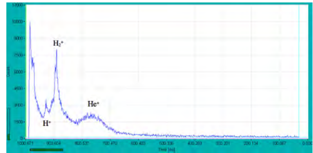
Figure 1.56: A time spectrum of after pulses showing H^+ , H_2^+ and He^+ contamination [31].
