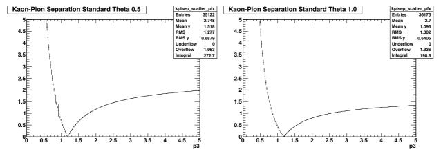
Now that K/pi separation and dE/dx resolution are simultaneously correct, the derivation of the "effective cluster counting" parameters is very constrained. If you look at my talk from the latest collaboration meeting or the previous DCH meeting, you can see the relevant equations. Basically the p2 and p3 are fixed to 1/2 and -1/2 by basic principles. The p1 parameter is given by
