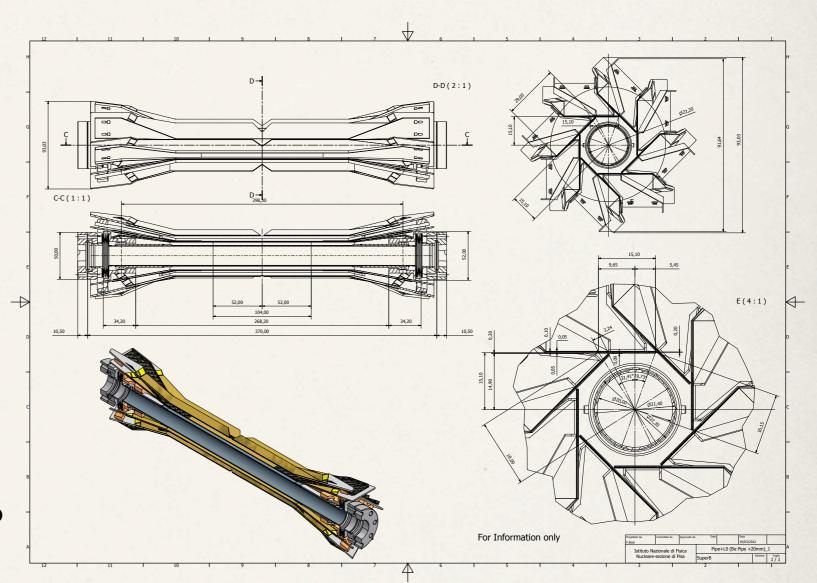
• Svt geometry for outer layers: outer layers are the same as in Babar, but SuperB acceptance is wider. Need symmetric fwd/bwd modules
