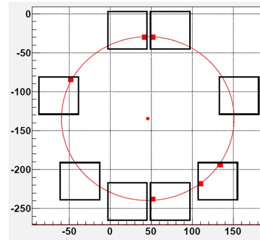
Ring reconstruction through fit of the PMT hits above threshold
