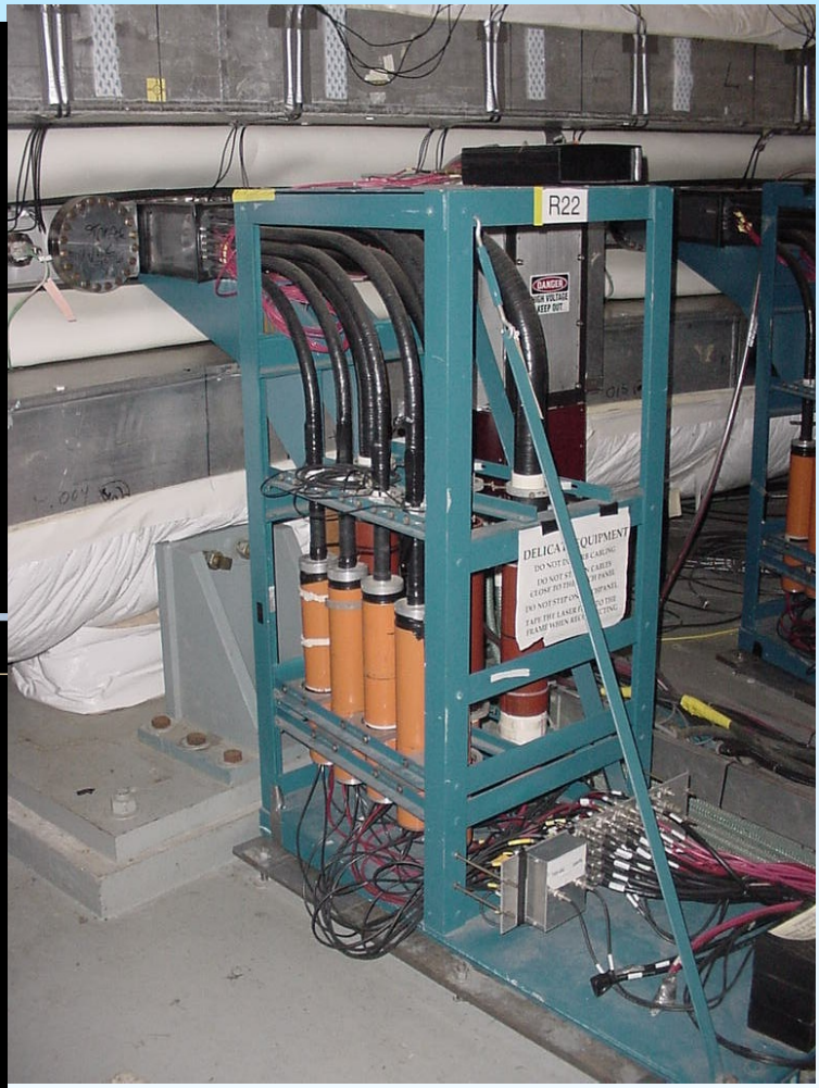
Picture of a Lead-Scifi Calorimeter from E821
