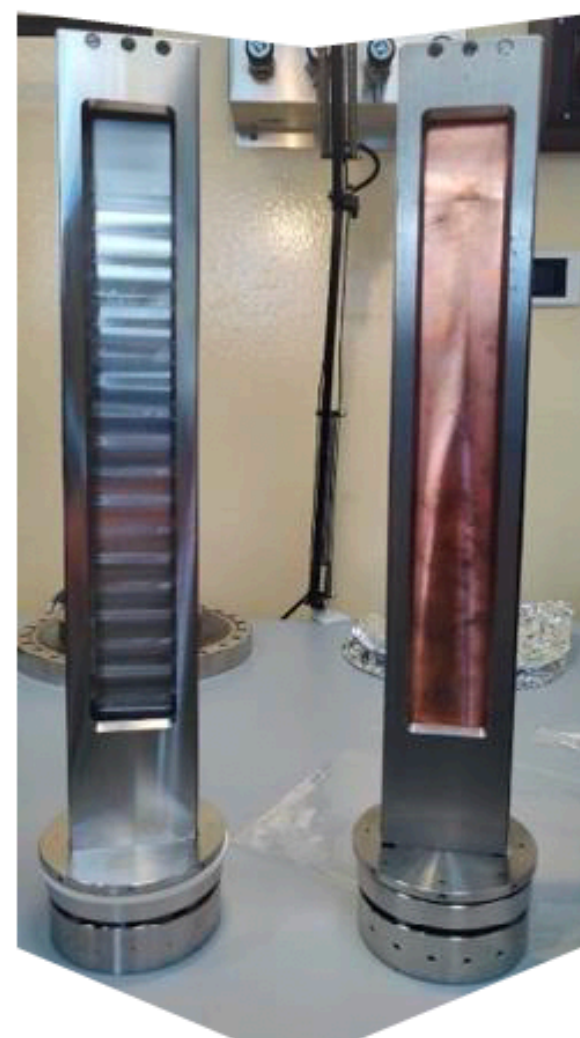
Rectangular Magnetrons for Nb 3 Sn 1.3 GHz coating system
