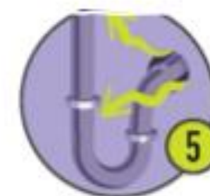
Gaps around service pipes
