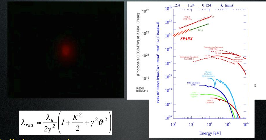
**Radiation properties: GW power - Monocromaticity - Tunability from IR to X– Short pulses**
