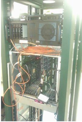
Fig. 3: The Vertical Slice at CERN. The AM board (right) and the EDRO (left) are shown inside the crate
