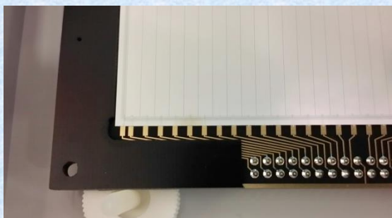
The strip side of a mounted prototype SSD
