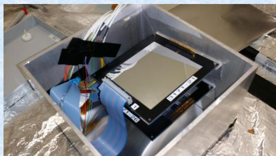
Two SSDs mounted in test enclosure
