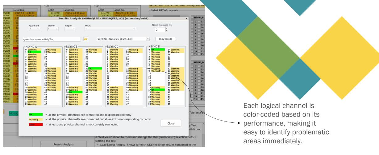
This panel (evolution of the already started "res" panel) provides a detailed visualization of the test results for a single ODE. By focusing on individual channels, the operator can precisely diagnose whether issues are due to noise, weak signals, or faulty connections.
