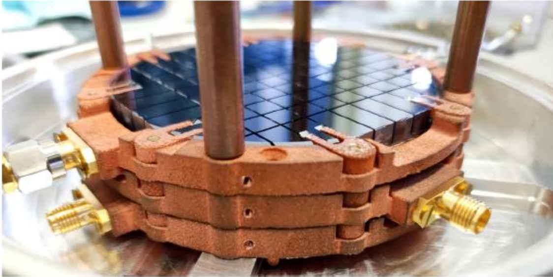
Figure 2. Top: Stack of 3 BULKID wafers as a proof of concept to scale the active mass of the detector. For the data acquisition and analysis described in this work only the top wafer has been used; Bottom: Map of the array used for the characterization of the background with lead shield. The master KIDs (red) trigger whole cluster, with the side units (blue) being acquired in coincidence to veto events. The resonators are numbered in order of increasing resonant frequency.
