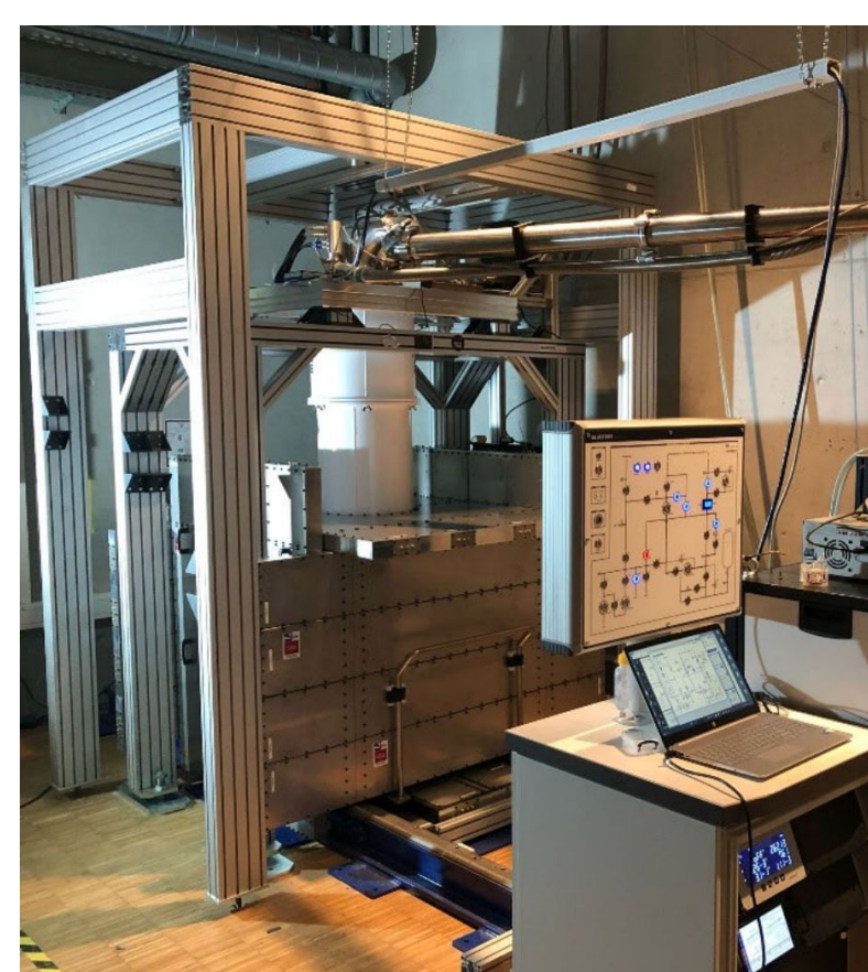
cryostat to keep the detector near the absolute zero
