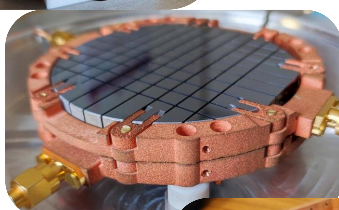
R&D on large wafer 50 g / 145 dice single 100 mm wafer first operations fall 2024
