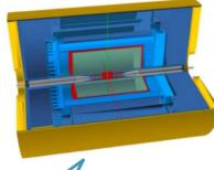
2) Particles hitting collimators are processed in BDSIM (G4 libs) to simulate interaction with material
