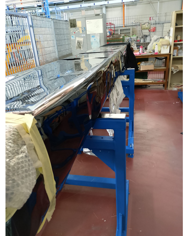
temporary light protection cover applied ⇒ to avoid possible ambient light irradiation of fibers
