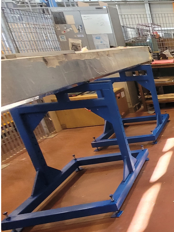
original tape wrapping partially damaged
