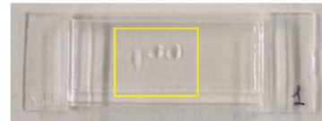
(b) Picture of the GelMA phantom. The three Ag-111 spots inside the yellow square are imaged.
