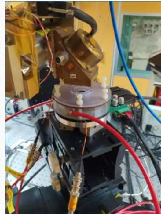
Prototype of GridPix detector at the Calibration facility at IAPS. Polarized X-ray source (X-ray tube and crystal scatterer) can be seen on the top to measure the response to fully polarized X-rays,
