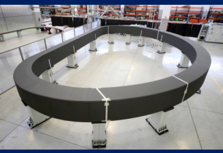
12. F4E | FUSION ITER TOROIDAL FIELD COILS France
