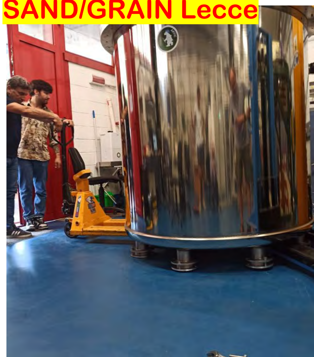
↑ ARTIC cryostat was previously lifted to allow the placement of the CRT bottom arm
