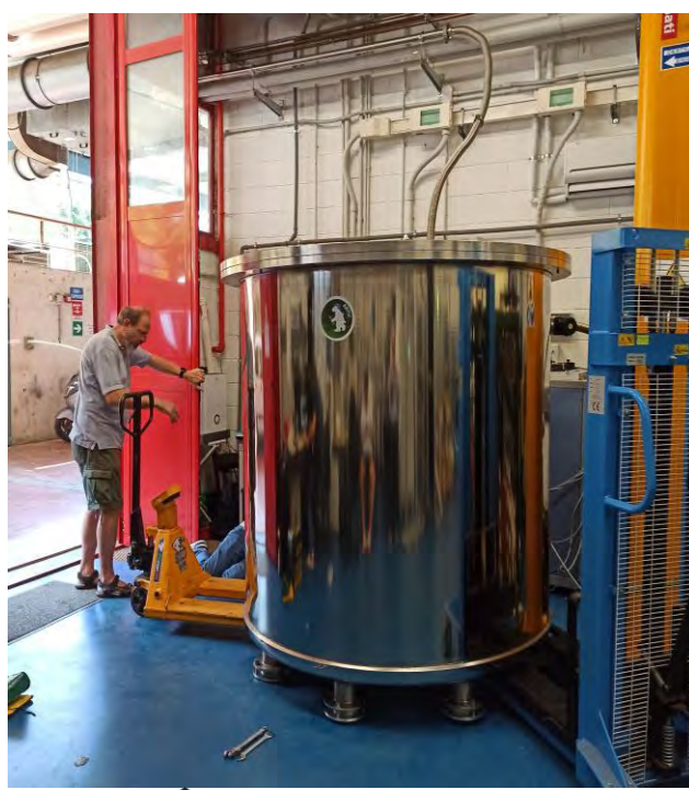
↑ ARTIC cryostat was previously lifted to allow the placement of the CRT bottom arm
