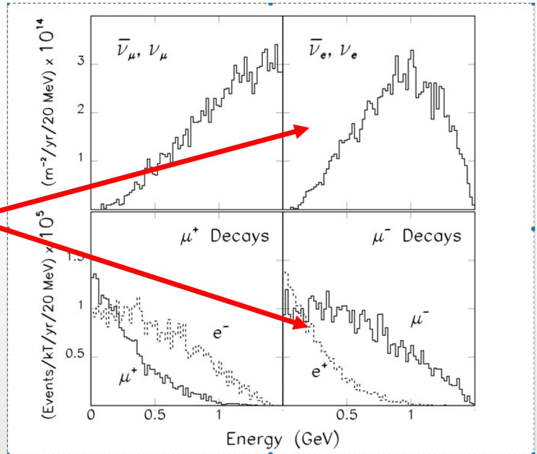
Calculated fluxes and spectra from a detector of 1 KTon, 1 km downstream of a muon source of 1.5 GeV/c for  $10^{21}$  p.o.t..
