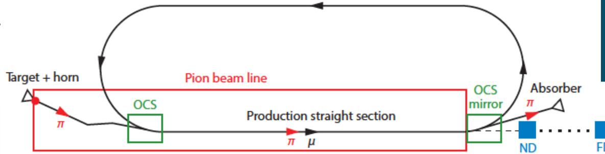
NuStorm as testbed for a stored muon ring
