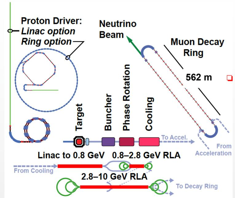
**Baseline: 10 GeV muons, one storage ring with detector at  $\sim 2000$  km, due to large  $\theta_{13}$**
