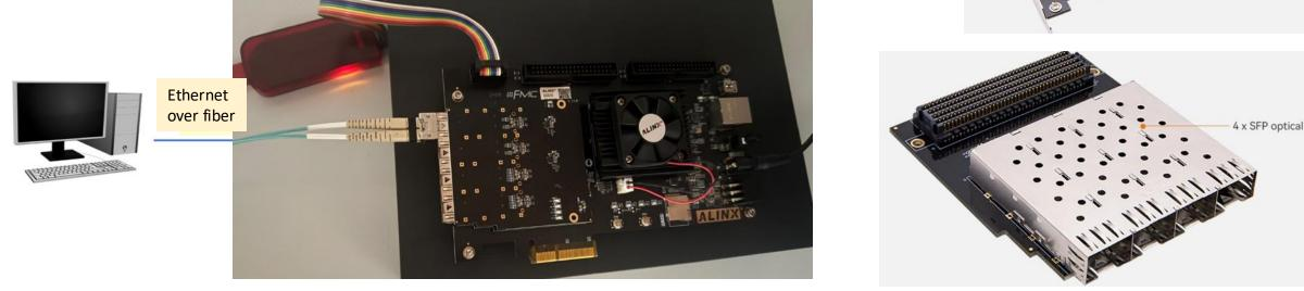
successfully implemented IPBUS communication over optical link (commercial SFP), first with GBIC SFP then with fiber: → configuration foreseen for test beam
