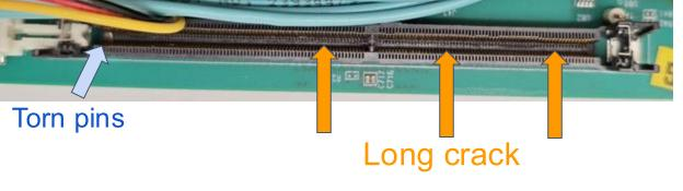
Repair not possible and card didn't boot (failed DDRMC) After many tests, workaround found: modified FW to bypass DDRMC and exclusion of ARM SoC (the one actually using DRAM)  $\rightarrow$  FLX-182 operational @RM1
