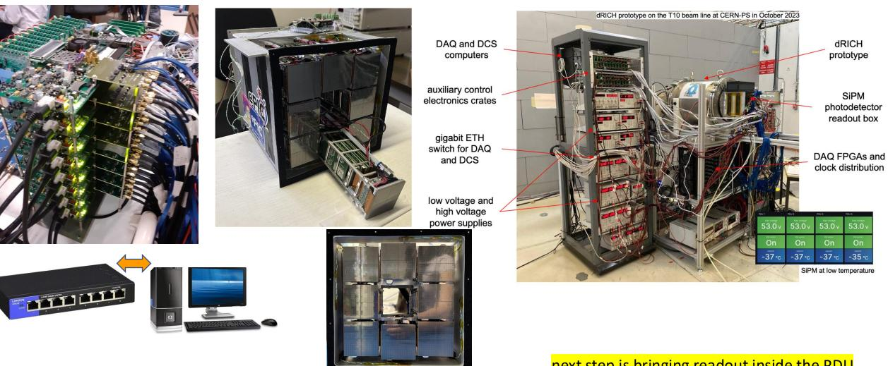
11 KC705 FPGA boards in parallel → 64 AlCOR chips → 2048 SiPMs next step is bringing readout inside the PDU (RDO comes after)
