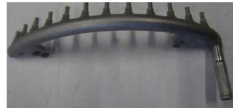
Orbital weldings between AM components and pipes
