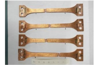
Figure 4-23: Room temperature samples after rupture test.
