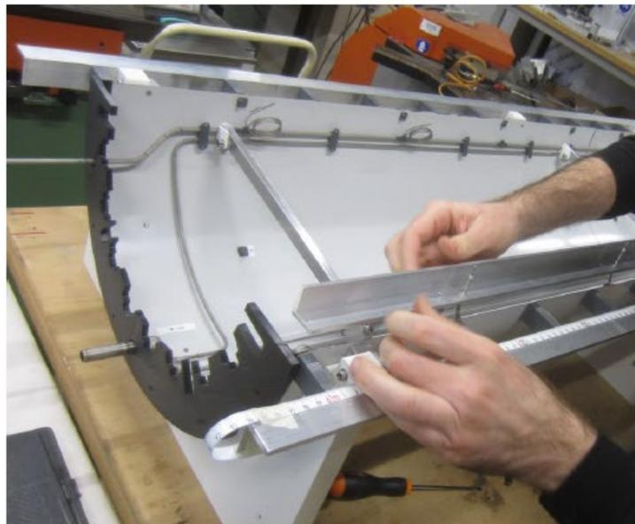
Positions of the fittings (for connection to the Half-Rings) is checked using a precision template
