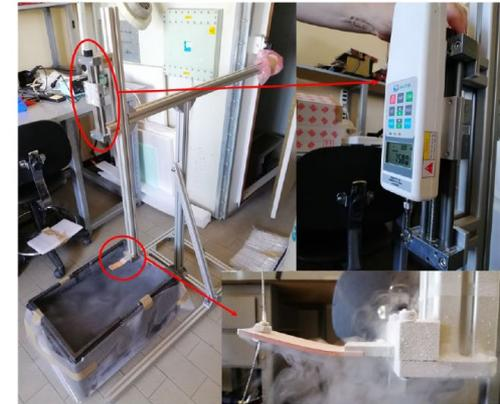
Figure 5-4: Test stand for the bending of the brazed samples, with a sample suspended above a LN2 bath. The top right insert shows the dynamometer in operating position. The bottom right insert zooms in on a bent sample: the connection point, i.e., the point where the pulling force is exerted, is clearly visible.
