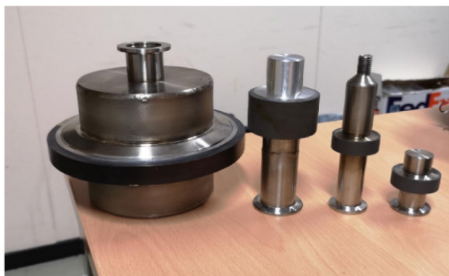
SMA-based UHV chambers with external diameters in the range 15-150 mm, DN16, DN25, DN100 pipe compatible. Heterogeneous joints (St/Ti, St/Alu, St/Cu)
