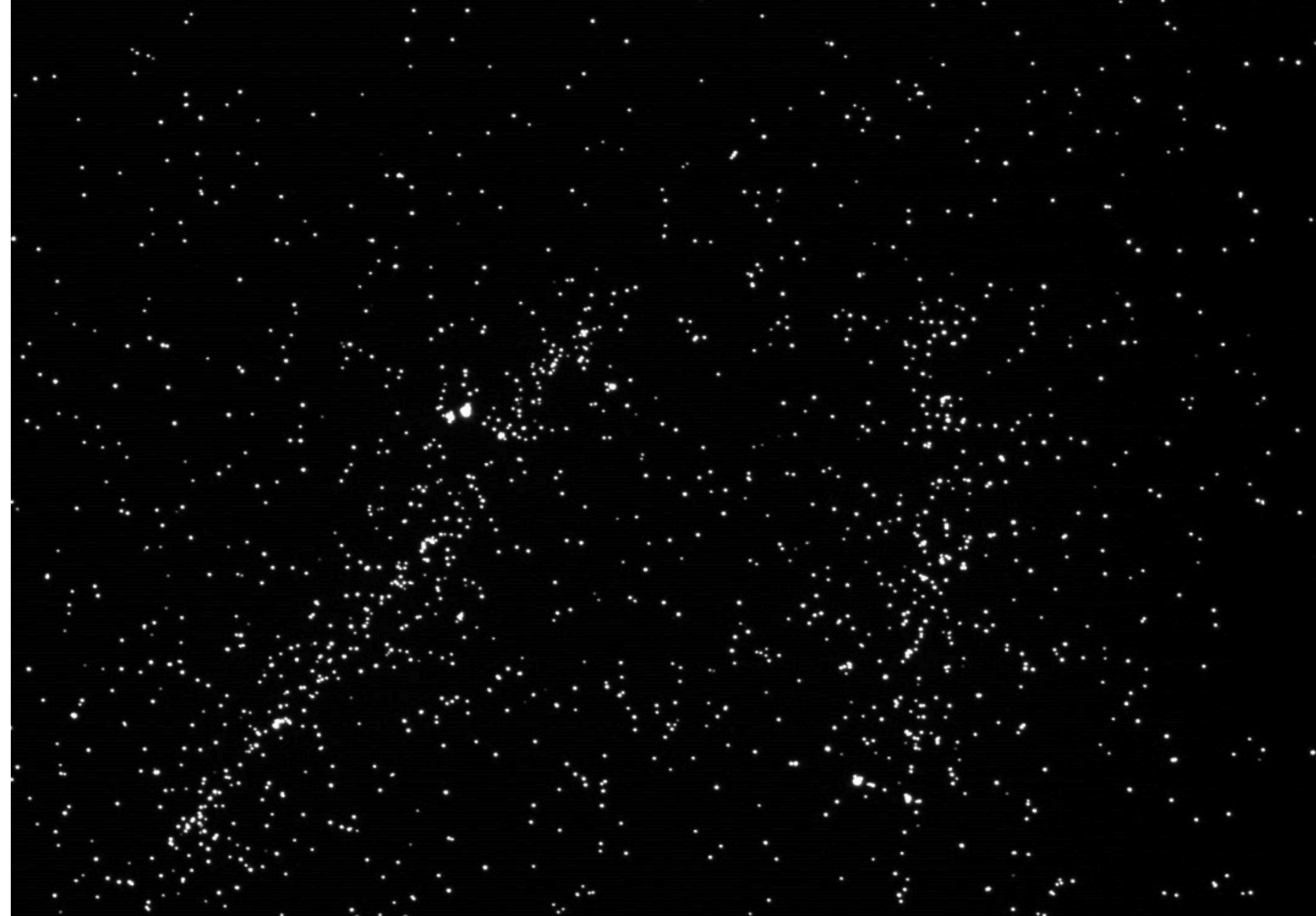
First image of a cosmic muon track passing through the CsI(Tl) scintillator. Two tracks are visible: the direct track and its mirrored image due to the reflection
