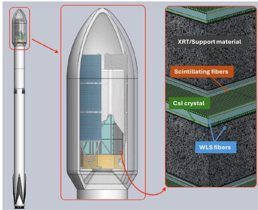
3m x 3m x 2.5m single module detector surrounded by an ACD made of plastic scintillators
