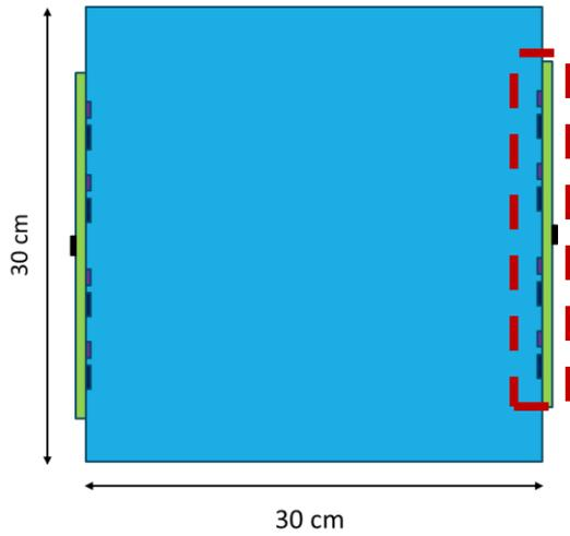
SiPM edge carrier boards with two SiPM sizes
