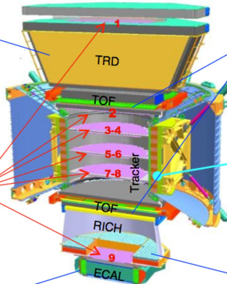
**The Charge and Energy are measured independently by several detectors**
