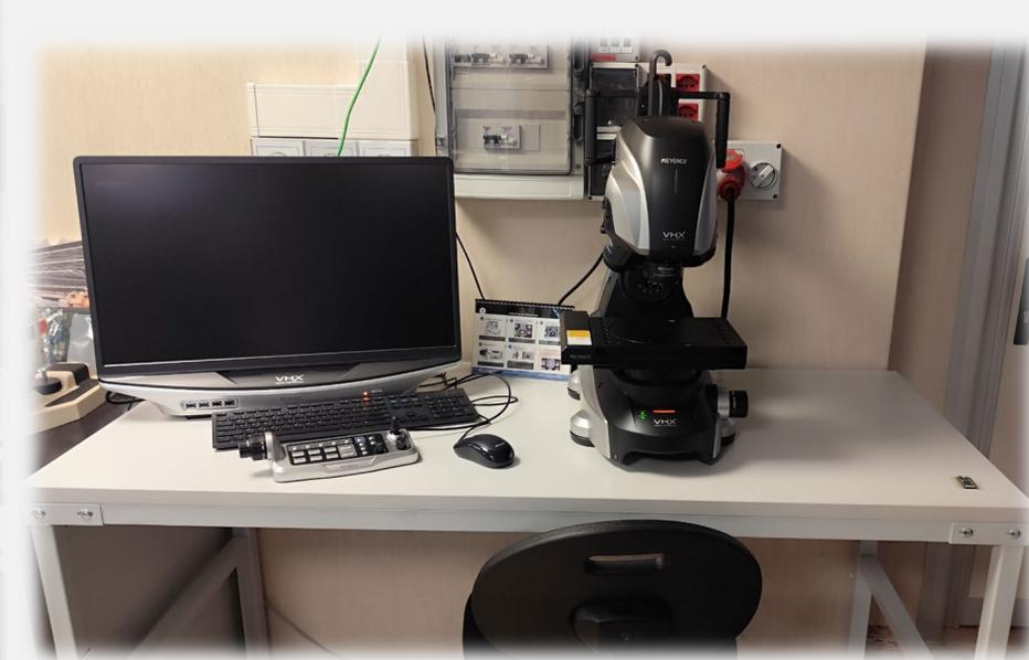
4K High Accuracy digital microscope capable of capturing high resolution images and measurement data for inspection and failure analysis
