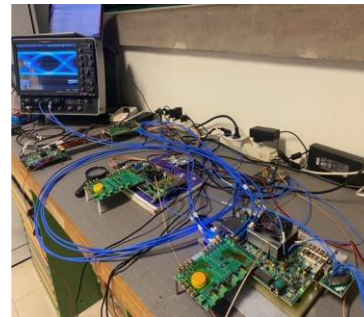
SER28_V1 Test Setup and Eye Diagrams (Eye Diagrams at 5,6,7 Gbps)
