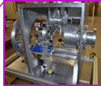
IRIS system built and tested at the SPES offline lab!
