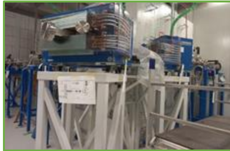
SPES Low Resolution Mass Spectrometer (WIP installation)
