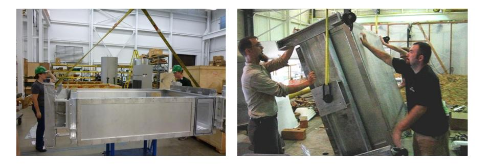
Motion Chassis and Hoist Beams work as designed. The TPC Enclosure can be lifted and rotated with relative ease.
