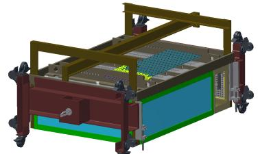
Configuration A Hoist beams bolted to TPC No relative motion TPC moves as one - simple lifting/ lowering
