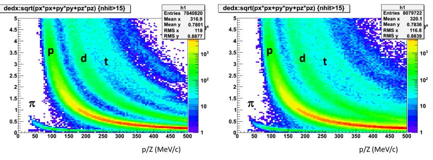
de/dx resolution pion@140MeV/c single:13.3% <-> min. bias: 16% proton@210MeV/c single:12.7% <-> min. bias: 14%
