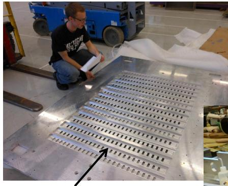
Holes for pad plane readout
