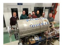
FNAL dipole demonstrator 14.5 T Nb<sub>3</sub>Sn
