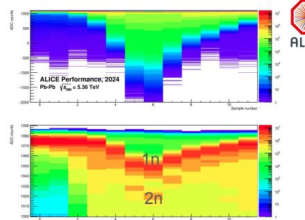
Energy resolution of ~16% is adequate to clearly separate neutron multiplicities 1n and 2n Possibility to precise calibrate the energy scale
