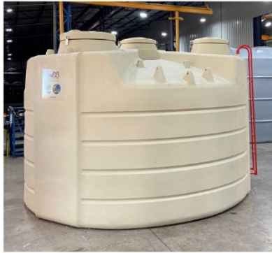
Figure 5: A prototype of a roto-molded HDPE tanks under consideration for the outer (low fill-factor) array.
