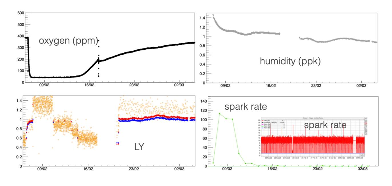
A study on filters effect, showed that a too low oxygen content, makes gas mixture unstable while high humidity has impact on the light yield;
