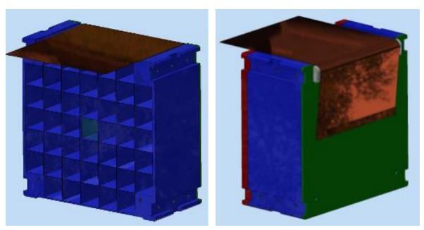
150 µm aluminum honeycomb foils for crystal housing and support (left) and detail of rigid-flex readout per layer (right)
