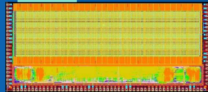
32x128 4k pixel matrix for beam test
