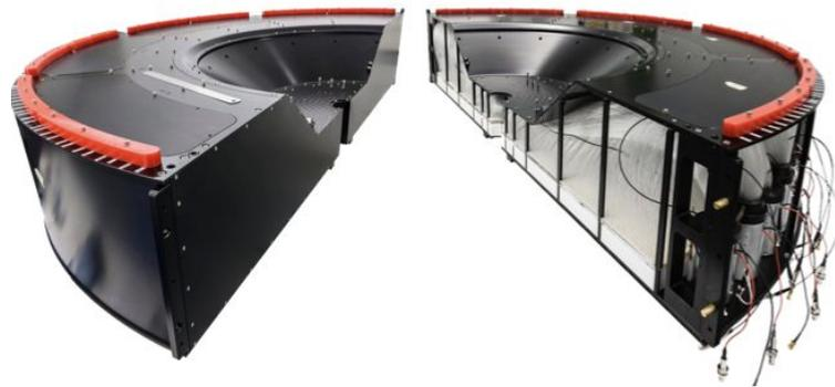
Two segmented scintillator disks for charged particle detect at  $4 < |\eta| < 7$ :
