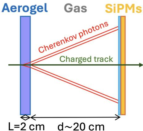
Target Cherenkov angle resolution achieved in test beam with small detector prototype
