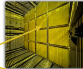
CPA-Cathode covered with TPB coated reflectors
