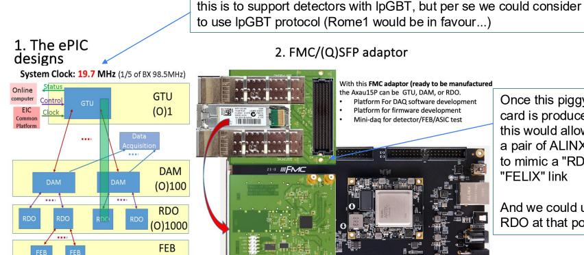
Mini DAQ, functionally includes GTU, DAM, and RDO Once this piggy back card is produced (by Jlab(, this would allow to use a pair of ALINX/AUX15P to mimic a "RDO" and "FELIX" link
