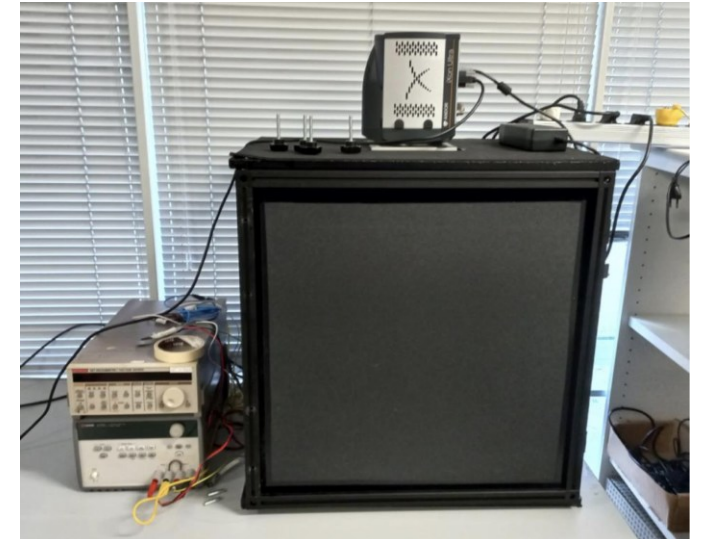
Andor CCD camera to detect the light emitted by SiPMs
