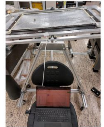
Wire tension measurements
