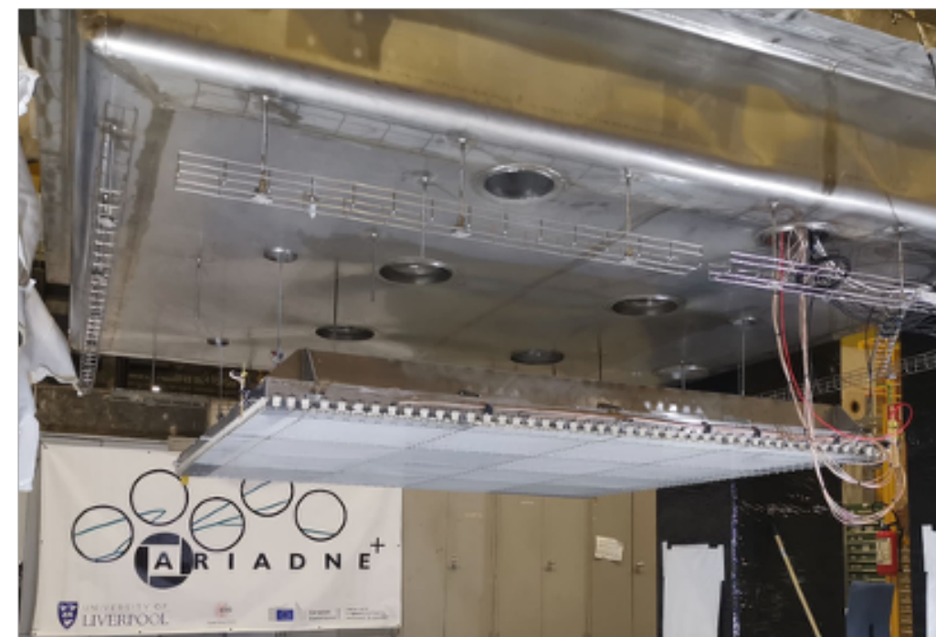
ARIADNE: Dual-phase optical charge (S2 produced in THGEMs) readout with fast cameras (TimePix3)
