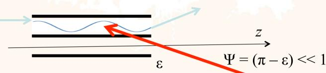
$$\omega = \omega_0 \cdot \frac{\sqrt{1 - \frac{v^2}{c^2}}}{1 + \frac{v}{c} \cdot \cos \theta} = -2\omega_0/(mc^2/E + E\psi^2/mc^2) < 2\omega_0 E/mc^2$$
