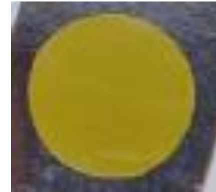
^{235}\text{U} target on Be substrate ( 25\text{ }\mu\text{m} ) March 2023, IJCLab Corentin Hiver PhD thesis, Université Paris-Saclay
