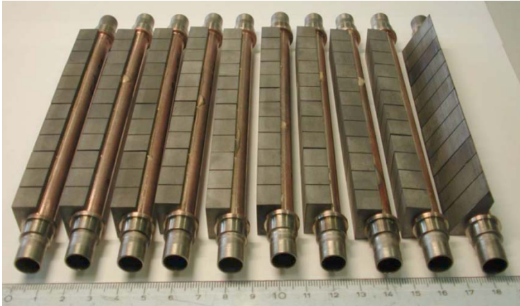
1. Be-tile brazed cooling pipes with Zr adapters
