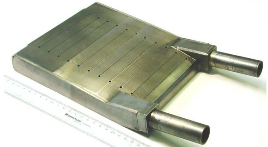
4. Half target after cover plates + joining pipes brazing
