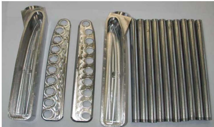
2. Zr cooling system manifold & collector plates
