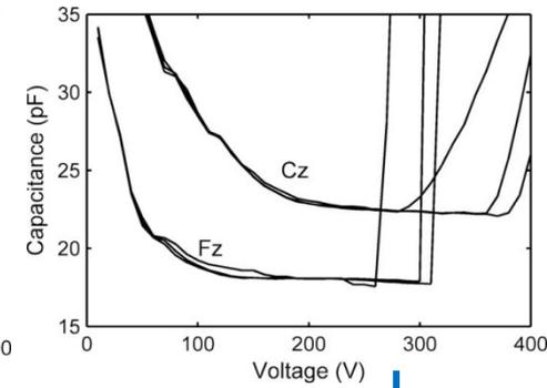
Characteristics of detectors at various times after 9 MeV proton irradiation: Cz (left), Cz & Fz (right)
