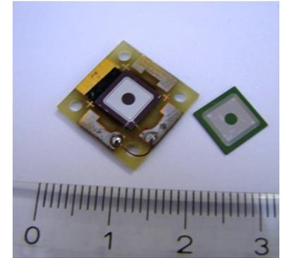
Processing (left) and mounting of silicon detector (right)
