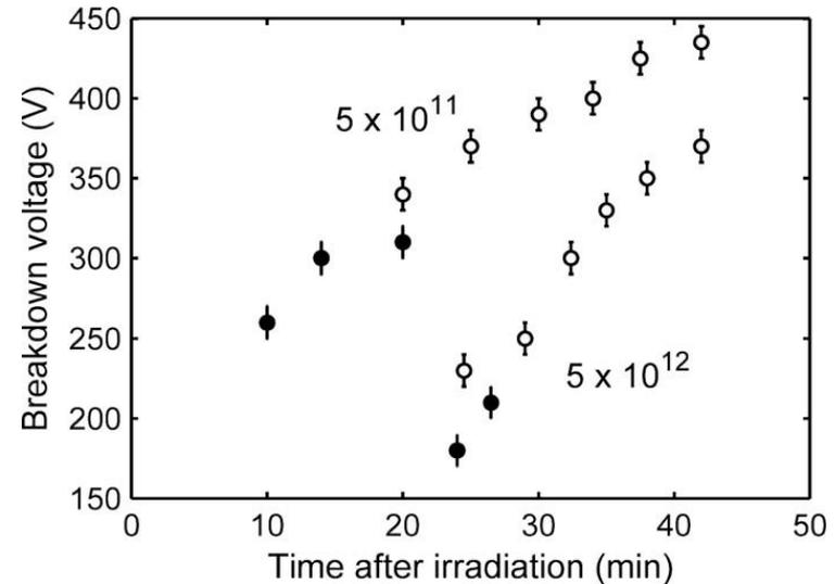
Recovery of breakdown voltage of the Fz detector
