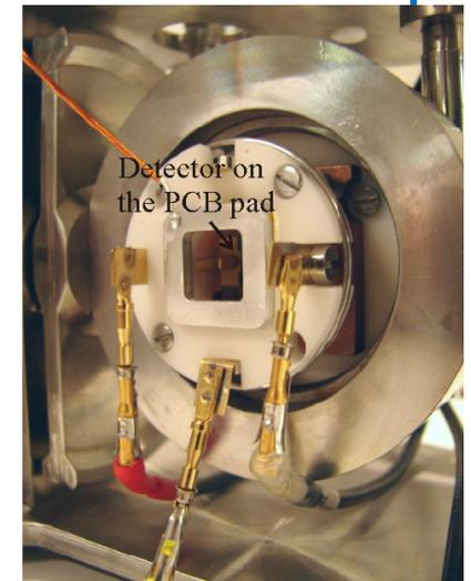
$LN_2$ -cooled goniometer for detector irradiation
