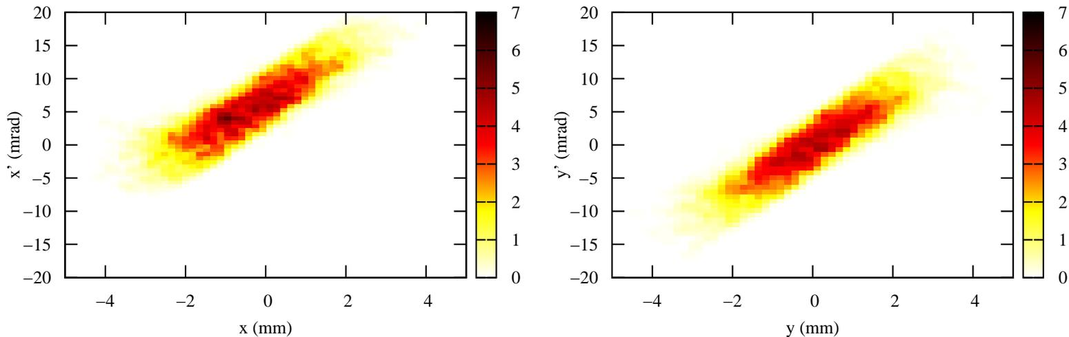
Beam exits the extraction with a 5 mrad angle. Can be corrected by electrostatic deflectors and/or dipole magnet of the injection beam line.
