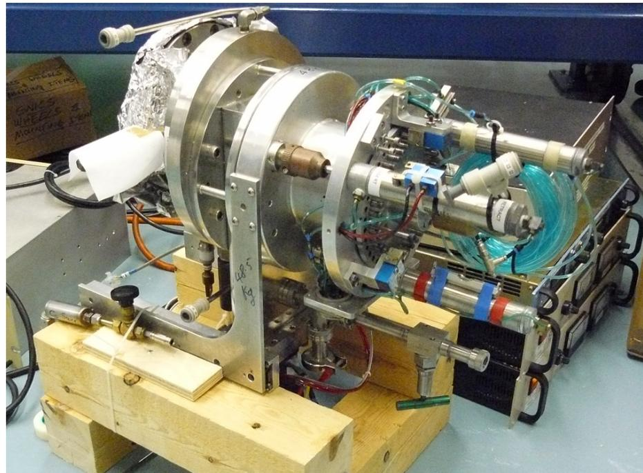
Second hand ion source from GNS, New Zealand is ready to be installed.
