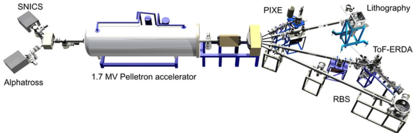
The applications would benefit from high brightness proton beams, that the existing Alphatross and SNICS ion sources couldn't produce.
