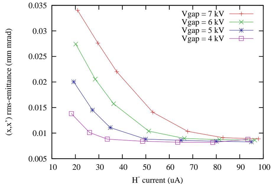
The minimum emittance value and location of optimum depends on plasma parameters, which are difficult to estimate  $\Rightarrow$  optimum has to be searched experimentally. Extraction is on threaded rods!
