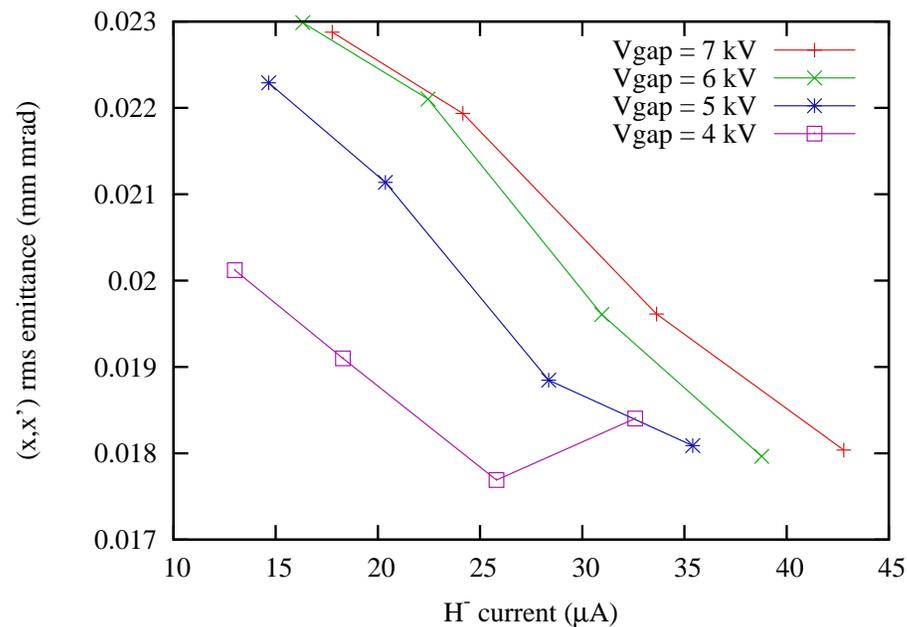
Extraction was designed for 100 µA current. Puller-plasma gap should be **increased** and/or plasma electrode aperture made **smaller** to reach optimum at typical current levels.
