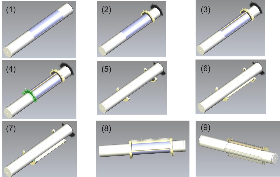
Tools under refinement after successful gluing. Mainly improving pressing components for longerons to the sensors.
