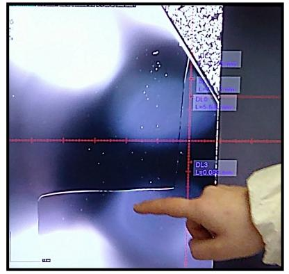
Crack stopped during bending procedures using microscope (not easily visible by eye).
