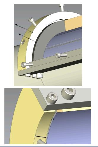
Increase the width of the holder  $\rightarrow$  To facilitate the alignment during the placement
