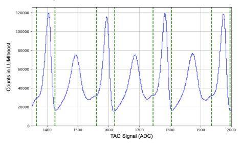
Signal selection through a cut on the time difference between trigger and event on CZT
